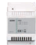
69RH Programmable device with 2 NO 3 A 230 V~ relays for 2 independent auxiliary controls
